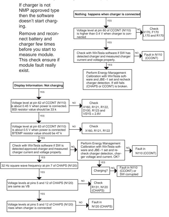
Figure 8. Trouble Shooting Diagram for Charging Failure
