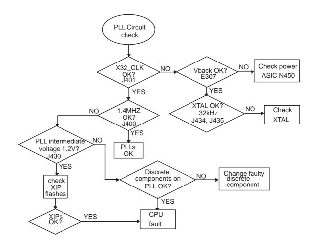
Figure 23. PLL clock generation circuit check
