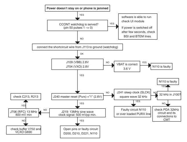
Figure 2. Trouble Shooting Diagram for Power Doesn't Stay On or phone is jammed failures
