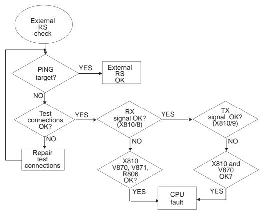
Figure 30. External serial connection troubleshooting diagram
