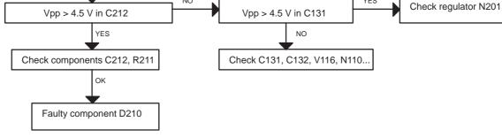
Figure 11. Trouble shooting Diagram for Flash programming doesn't work (via system connector X170)
