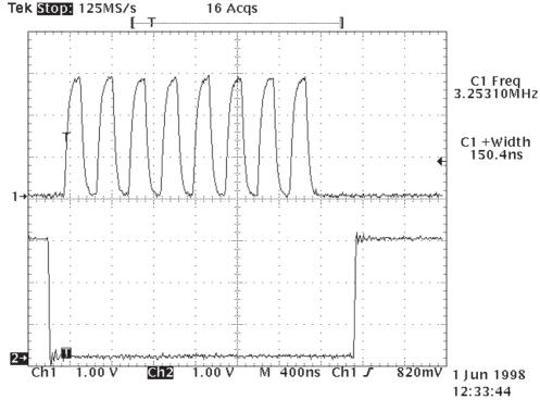
Figure 37. GENSCLK (J706) and LCDCSx (pin 5/H700) , LCD active after pressing a key.
