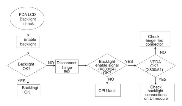
Figure 27. PDA LCD backlight troubleshooting
