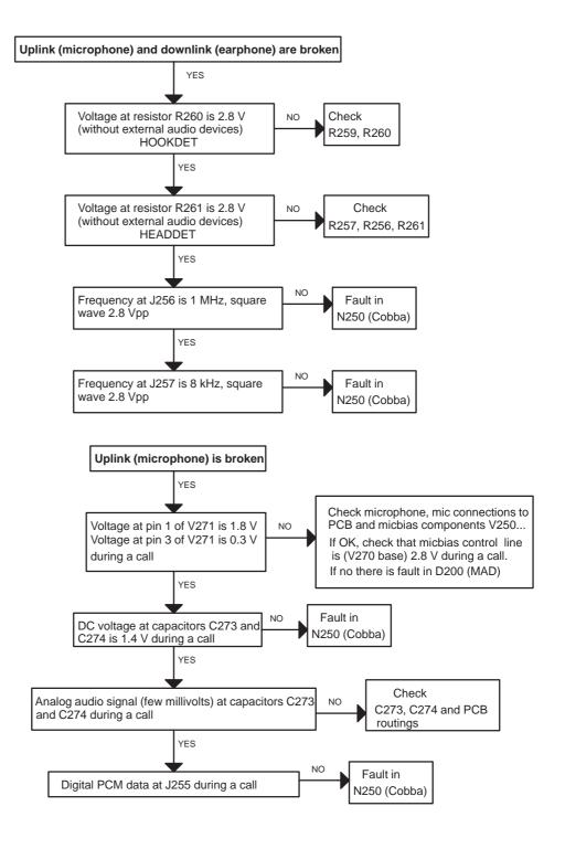
Figure 6. Trouble Shooting Diagram for Audio Failure
