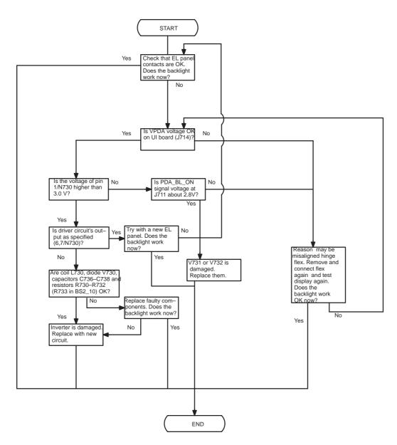
Figure 47. Flowchart for troubleshooting of the PDA backlighting circuit.
