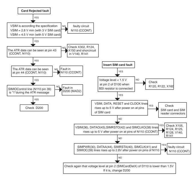
Figure 5. Troubleshooting for SIM card faults
