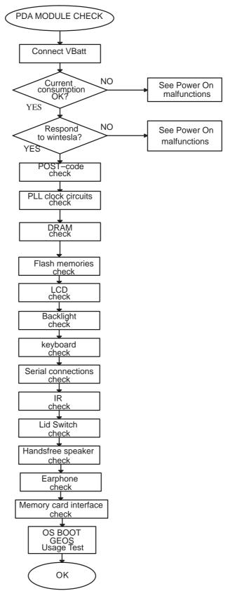
Figure 20. The highest level of the PDA troubleshooting diagrams
