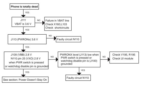
Figure 1. Trouble Shooting Diagram for Phone is totally dead failure
