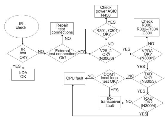
Figure 31. IR connections troubleshooting diagram
